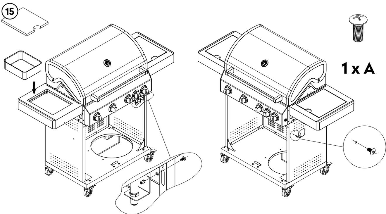
The gas distributor is attached with a cable tie below the console for transport. Untie the cable tie and attach the gas distributor to the side panel.
